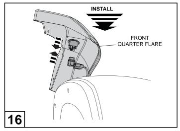
Hold fender flare assembly close to the bumper & fit Active park assist sensor to the escutcheon as per the Ford Workshop Manual (note the audible 'click' when the sensor is fully home).
