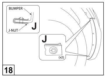
Hold the splash guard inwards and push the supplied (2) J-nuts onto the front bumper in the top and bottom hole position as shown.
