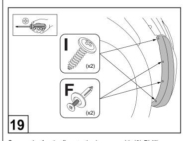
Secure the fender flare to the bumper with (2) Phillips head screws and (2) scrivets as shown.
