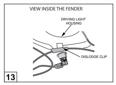
Follow the wiring harness that supports Active park assist sensor up to the edge clip located under the driving lamp assembly – dislodge the edge clip from the bumper & leave off permanently.
