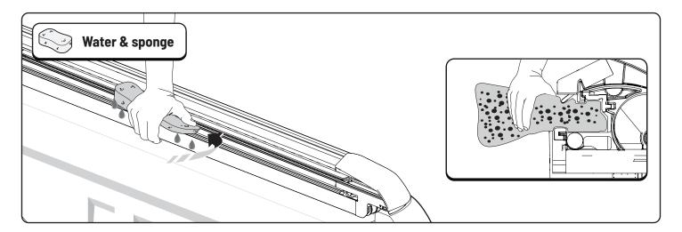
• Clean the drainage channels on the side profiles. Do not use high pressure cleaner.
