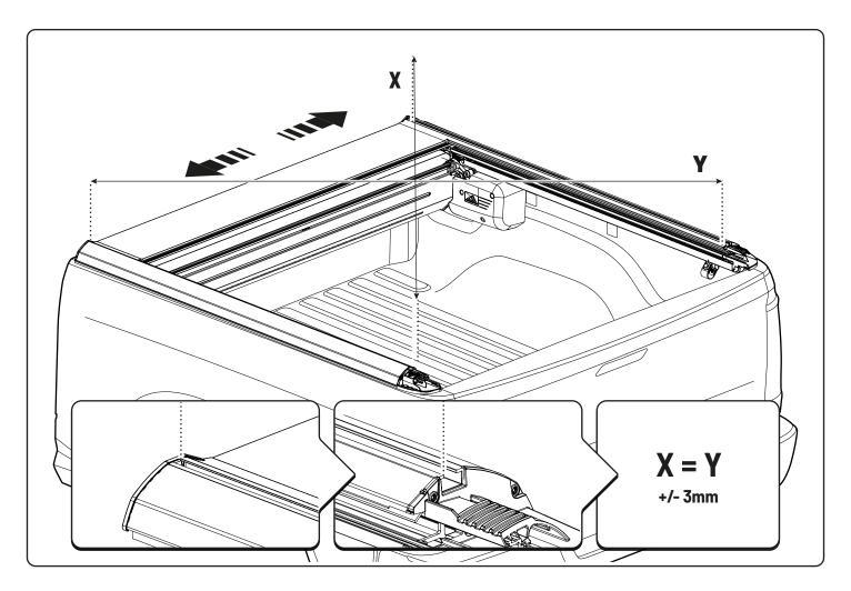
• Ensure the cross measurements are identical.
