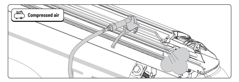
Remove dirt and debris using compressed air.
