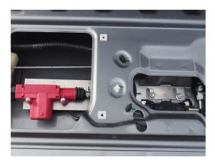
2) Remove the two screws that hold the tailgate handle into the tailgate
