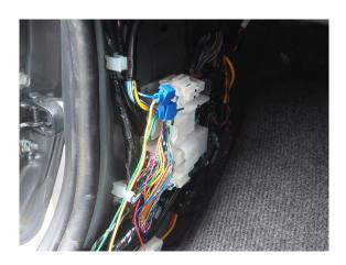
8) Connect the Central locking kit into the vehicles Central locking Loom
