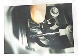
22) Close the clip onto the rod. Ensure that the threaded part sits across the full width of the clip
