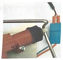
14) Thread wiring loom into tailgate
