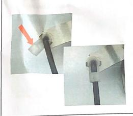
13) Connect wiring loom to the mechanism
