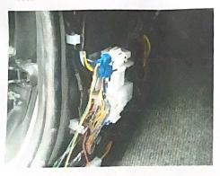
**26)** Connect the central locking kit into the vehicles central locking loom
