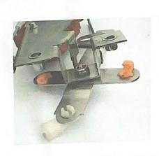
12) Push the handle actuator rod into the clip and close the clip onto the rod
