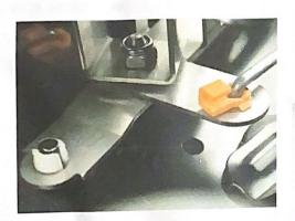
**18)** Bolt the Eagle actuator kit to the tail-gate using the screws and shake proof washers removed in step 6
