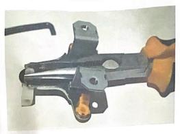
11) Push clips into Eagle actuator kit as shown
