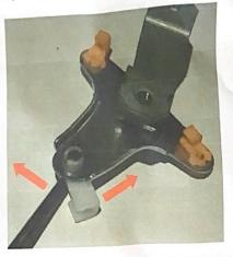
10) Remove white and orange clips from original mechanism by carefully squeezing clip tails together with pliers or with fingers. Push clip out of mechanism
