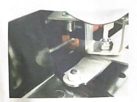
17) Connect the nearest tailgate rod into the clip and close the clip onto the rod
