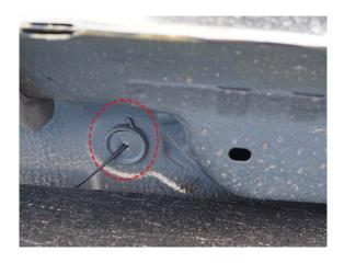
11) Remove door sill guard on drivers side, to gain access to vehicles wiring loom
