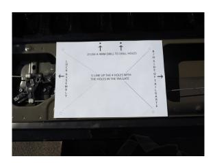
5) Drill Holes to mount the motor. Please use a 4mm drill piece
