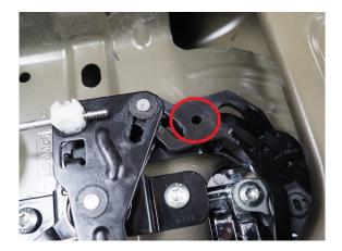
2) Drill a 4 mm Hole in the centre of the lock mechanism (see picture)
