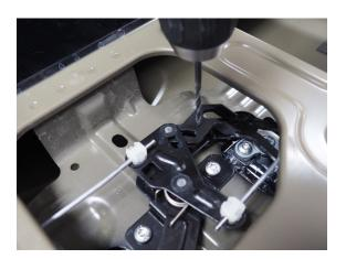
4) Use the template provided to mark holes required to mount the Motor
