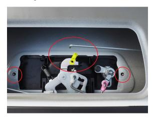
4) Disconnect the Rod from the back of the key barrel and remove the pink plastic clip
