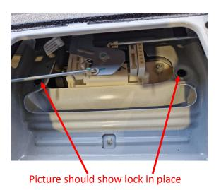
**10)** Feed the wiring loom into the tailgate and attach the loom to the actuator
