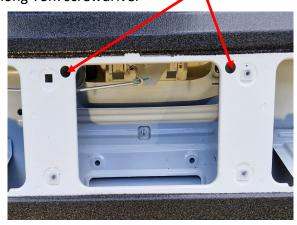
**6)** Remove the two screws that hold the tailgate handle in place
