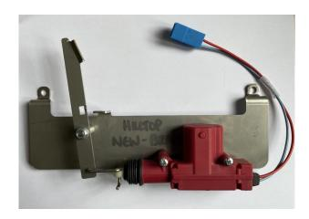
**8)** Position plate and actuator with the fixing legs over the tailgate handle holes, threading the actuator arm underneath the tailgate lock rod
