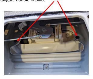
**7)** Place the actuator arm in the unlocked position
