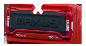
**4)** Open tailgate; undo 12 screws to remove metal panel as highlighted
