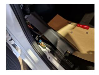
**13)** Route the cable from the tailgate along the chassis, into the body and to the kick plate
