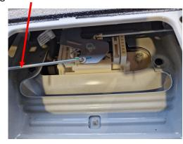
**9)** Replace and tighten the tailgate handle screws to secure the base plate
