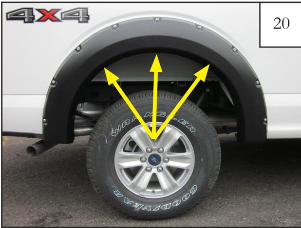
20 Press flares firmly onto the vehicle and install and fully tighten three screws (SW1-0050) into the clips installed in step 18.
