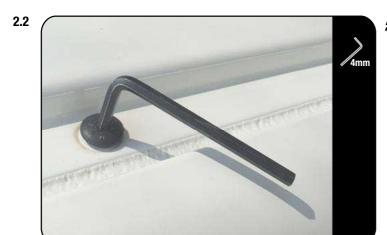
Use a 4mm Hex Allen Key to remove the above bolts from the roof channel.
