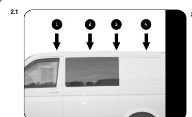
If you are installing a Full Rack remove all the OEM Plastic Button Head Bolts, but if you are installing a Half Rack remove the rear Bolts (3 & 4) on the left and right hand side of the vehicle.
